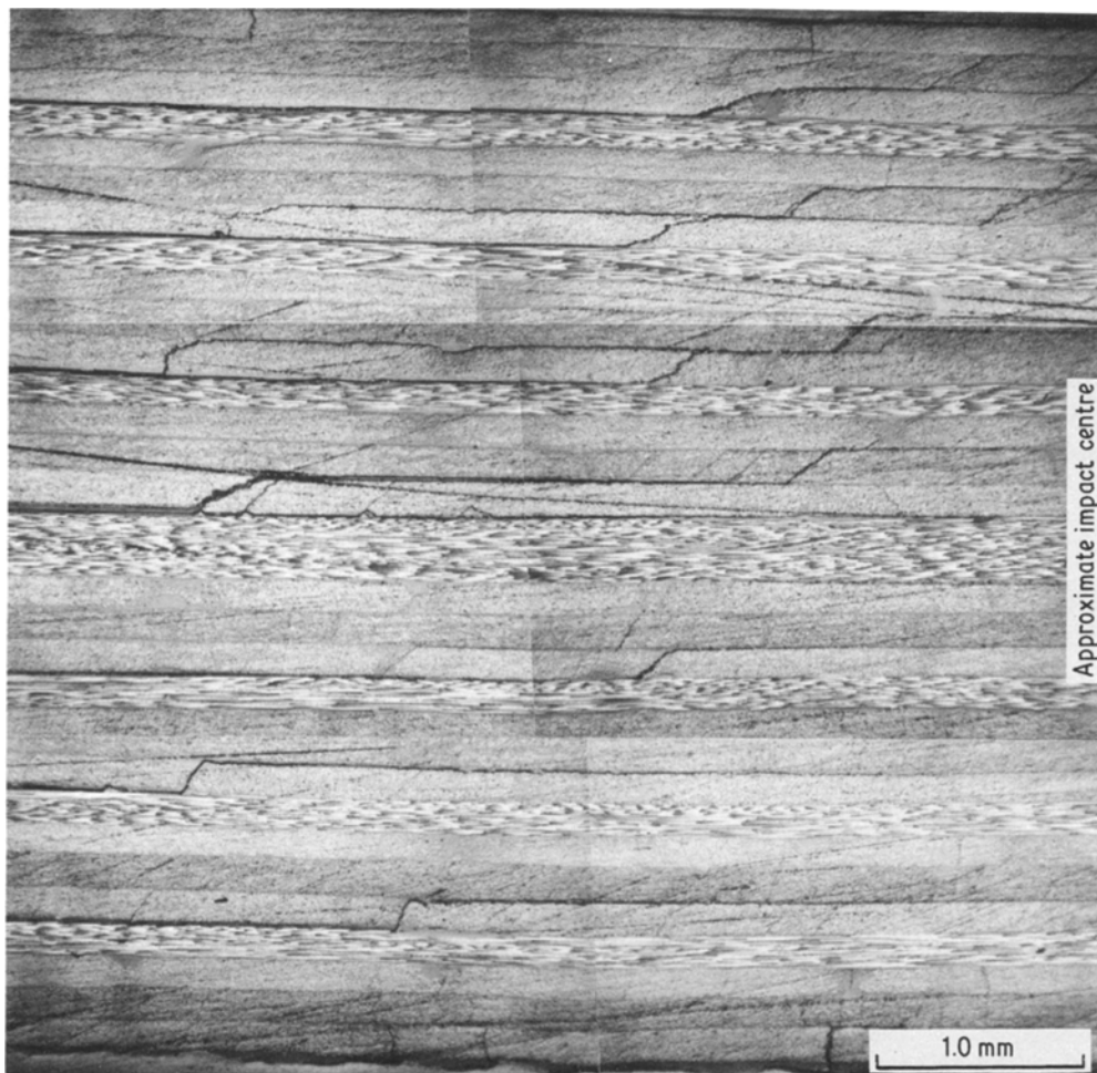
Figure 4 Impact damage in 3501-6/IM7G.
