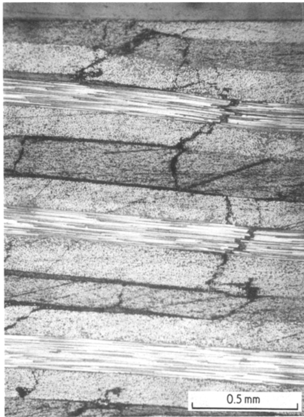
Figure 10 Transverse cracking in 8551/IM7G.
