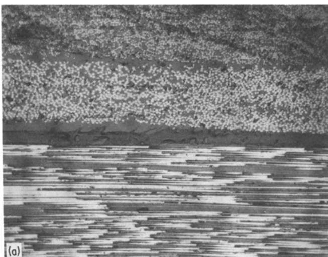
Figure 8 (a, b) Resin tearing associated with delamination of 3501-6/IM7G.
